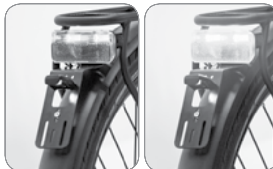
Holding the brake lever will make the rear light shine brighter
