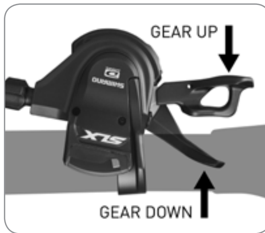
Rapidfire shifter control of the derailleur gears
